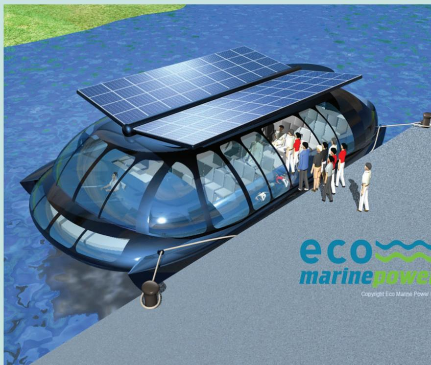
**Impression of the eco solar ferry concept Medaka. The solar panels mounted on the roof are used to recharge batteries to help reduce fuel consumption and noxious gas emissions.**
